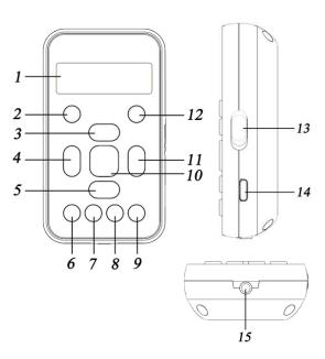
1. **LCD DISPLAY** 2. **POWER** 3. VOL+ 4 TUN- << 5. VOL-6. PRESET 7. PRESET NUMBERS 1 & 2 PRESET NUMBERS 3 & 4 8.
