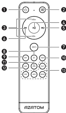
1. button ---- Switch the unit between On and Standby mode.
